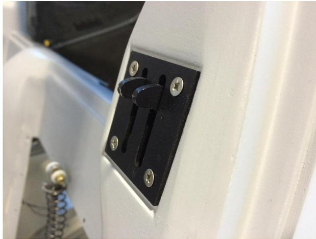
Photo of Canopy Latch Claws Modified to Remain Partially Extended
