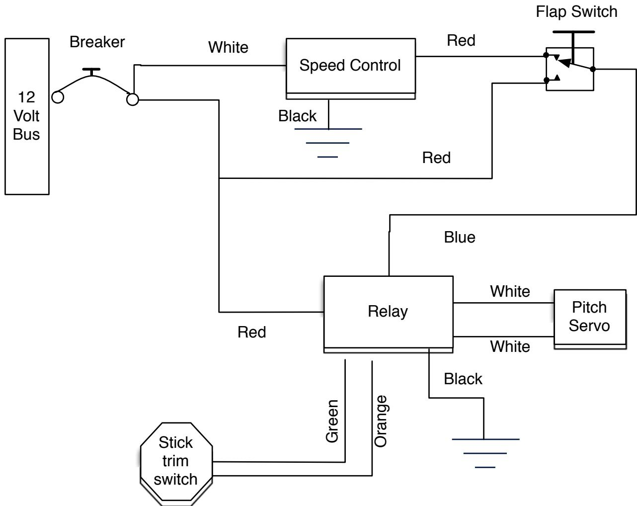
Flap (or airspeed) switch wired so that when flaps are up blue relay line gets 12v power, when flaps are down blue relay line gets power from speed control.
