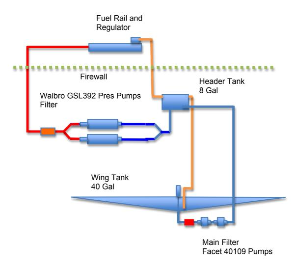
Fuel is drawn from main (wing) tank filtered and pumped via two 40109 facet pumps in series (Pri and Sec) to Header Tank Some 18inches above.
