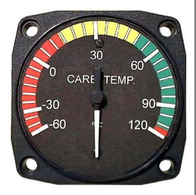
There are many instruments available that can give the pilot carburetor temperature information, many of which are non-TSOd "stand-alone" units for the amateur-builder, in addition to these single instruments (such as those made by Westach) there are several engine information systems (EIS) such as those offered by Grand Rapids, Rocky Mountain and Dynon that offer the option to monitor carb temperature and even include alarms.
