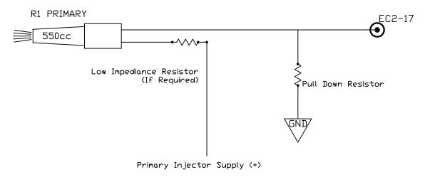
Alternate 1 - Low Impedance Resistor Location
