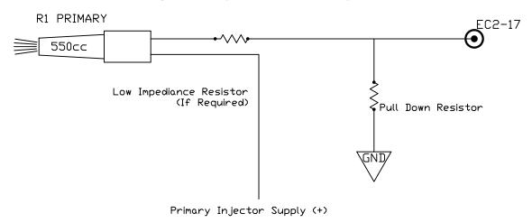
Alternate 2 - Low Impedance Resistor Location
