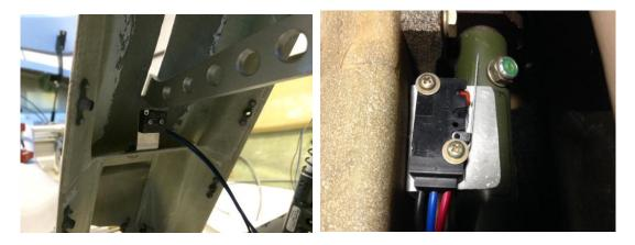
Canopy latching lever micro switch mounting examples
