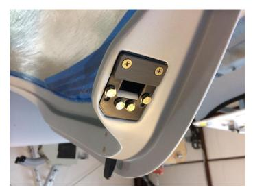
Photo of Canopy Striker Modified with Lift Plate Installed
