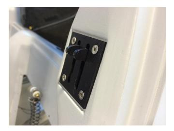
Photo of Canopy Latch Claws Modified to Remain Partially Extended When In Full Canopy Release Position
