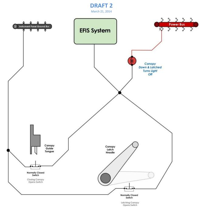
Canopy Safety Warning Wiring Drawing Example
