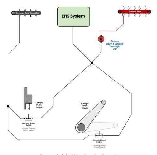
Canopy Safety Wiring Drawing Example
