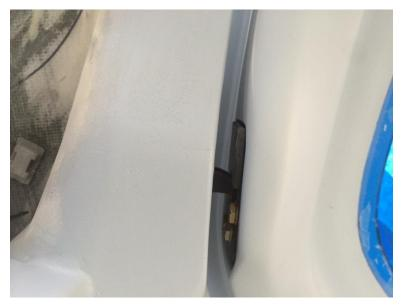
Photo Showing Claws and Striker Plate with Canopy Propped Open by Latch Mod
