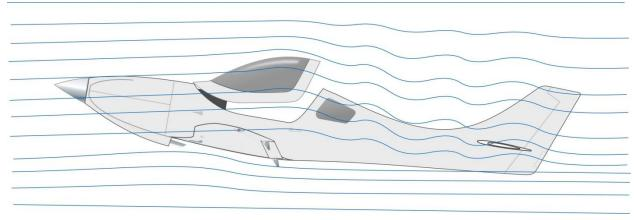
Illustration of disturbed air flow with canopy open
