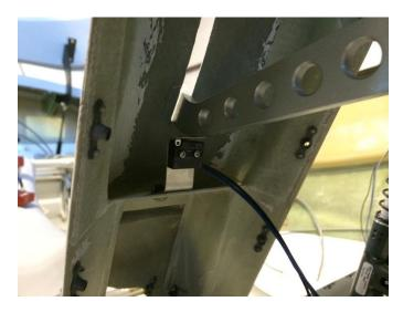
Canopy latching lever micro switch mounting example
