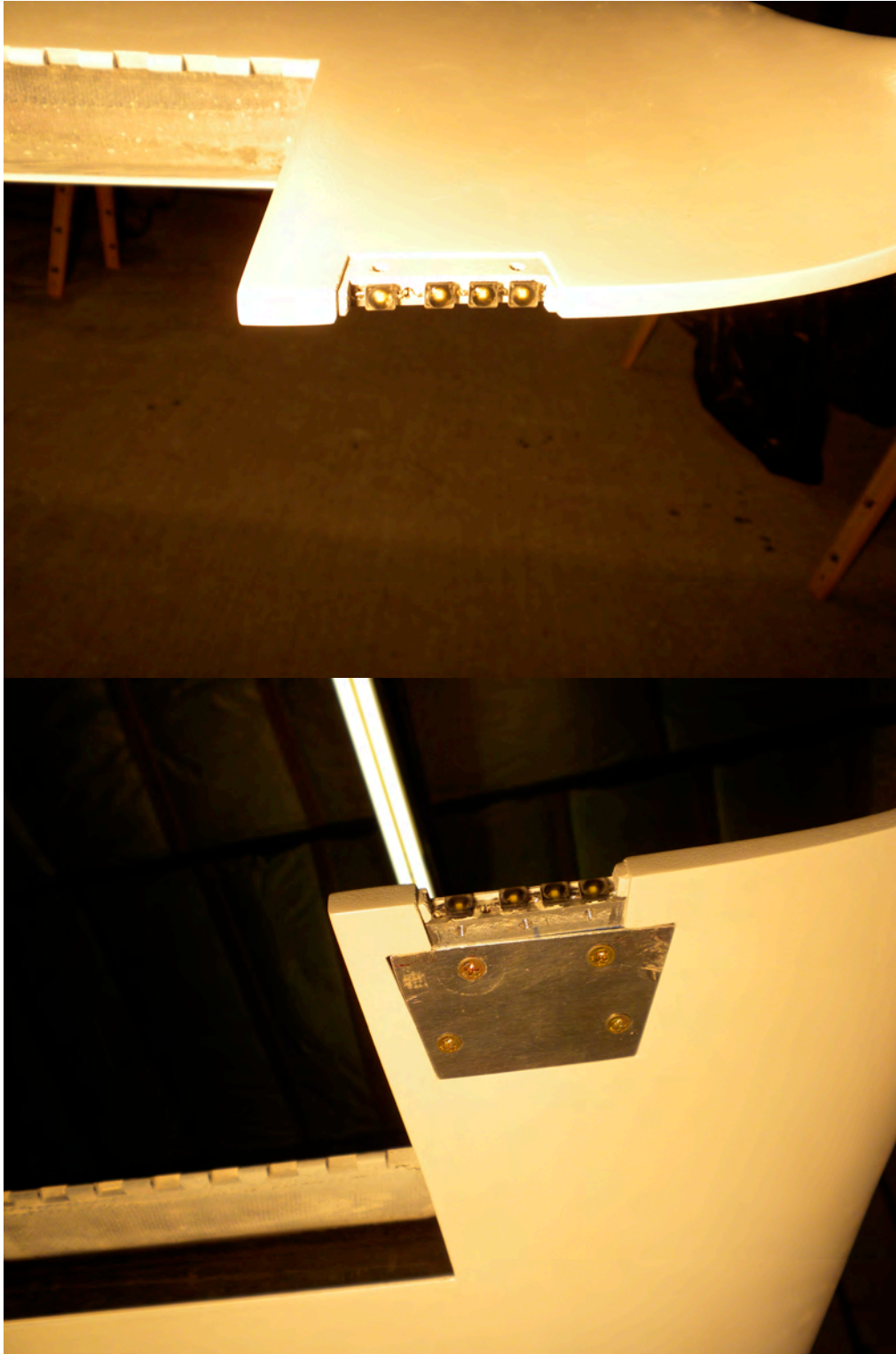
Rear facing LEDs. The three on the right are the strobe LEDs. The one on the left is the position light. All four are glued to an aluminum block. The bottom frame shows the block and a larger area heat sink attached to it on the underside of the wing.
