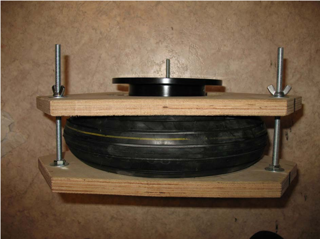
Side view of tire changing tool compressed
