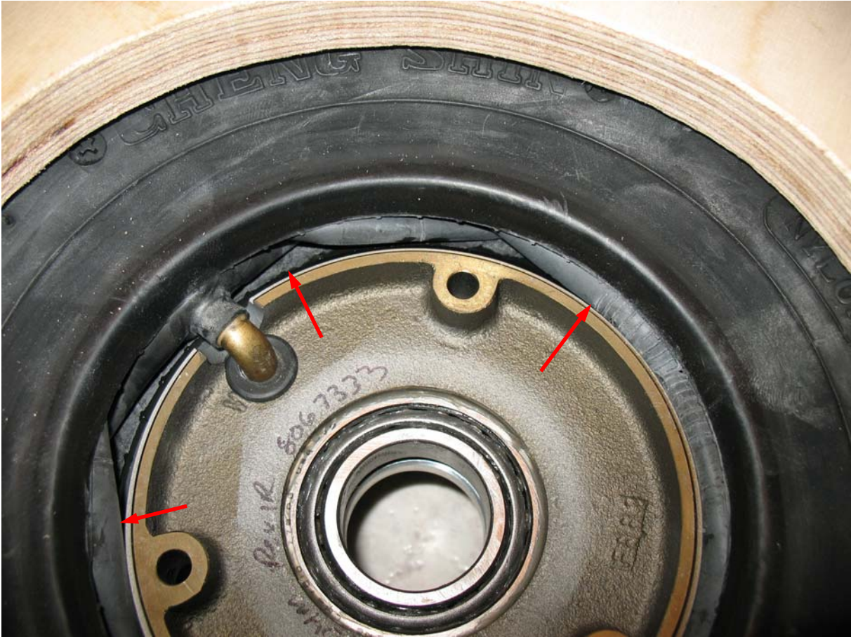
Adjust tube accurate to stay out of rim intersection area
