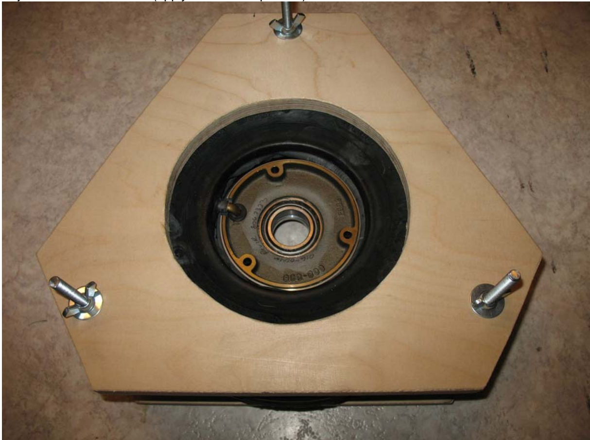
Fill little air to tube for better adjustment (not too much); apply part two of the tool and tear down
