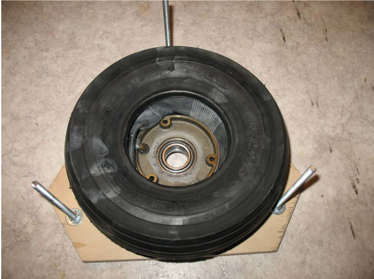
Adjust tire and insert tube (apply little talcum powder)
