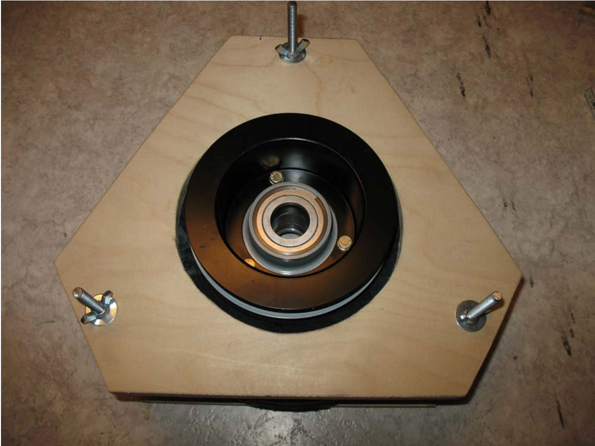
Apply brake disk (here: Groove type); Apply rim bolts and torque
