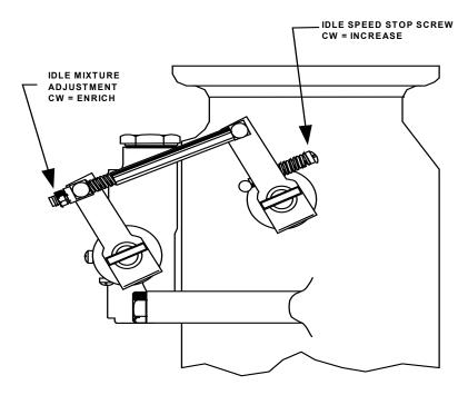
FIGURE 8 - THROTTLE & CONTROL ASSEMBLY SIDE VIEW (EXCEPT GTSIO-520-D, F, H,, K, L, M, N)
