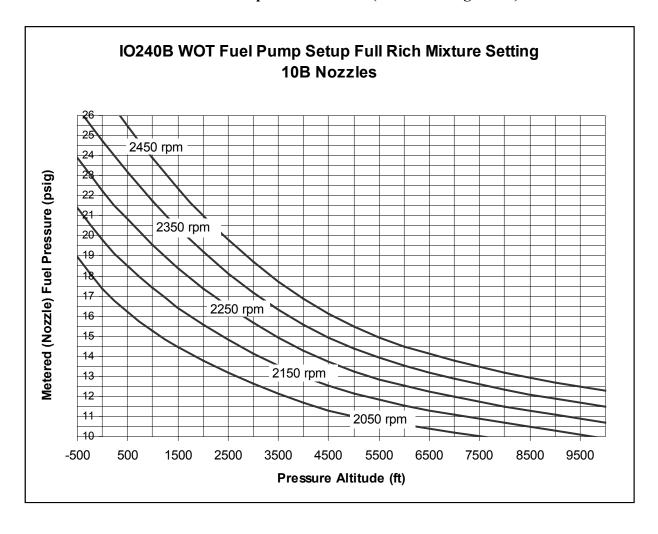
NOTE: At conclusion of setup, reset the idle speed to 850 RPM (+/- 25 RPM) and verify idle cutoff mixture rise, acceleration / deceleration without excessive idle speed dip, and idle stability.
