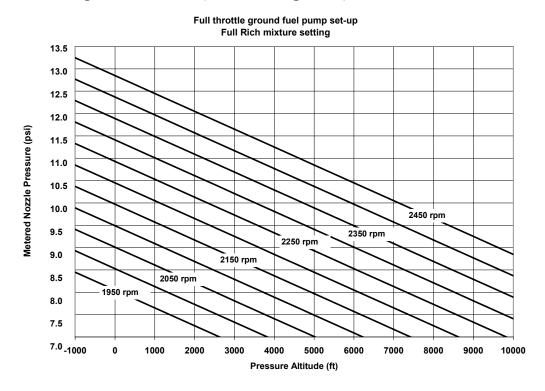
NOTE: At conclusion of setup, reset the idle speed to 850 RPM (+/- 25 RPM) and verify idle cutoff mixture rise, acceleration / deceleration without excessive idle speed dip, and idle stability.
