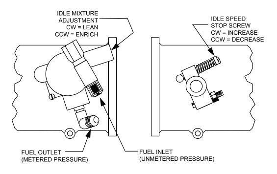
FIGURE 6 - THROTTLE & METERING ASSEMBLY
