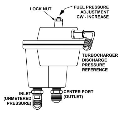
FIGURE 10 - FUEL PRESSURE REGULATOR FOR TURBOCHARGED ENGINES
