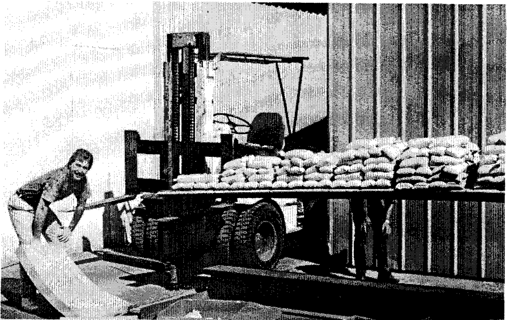
Figure 11.1. Structural Testing of the LANCAIR IV Composite Wing
