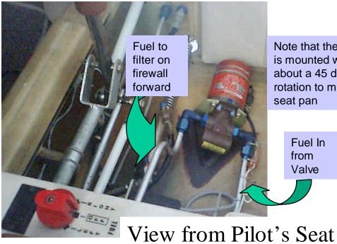
Note that the pump is mounted with about a 45 degree rotation to miss the seat pan
