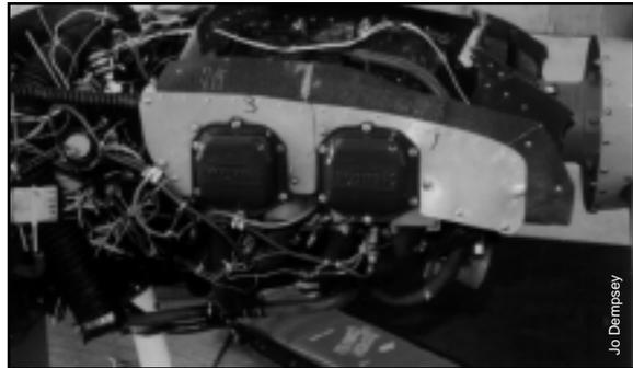
the ground. During the pre-takeoff run up it is difficult to tell any difference between operation on either ignition. The RPM drop is virtually the same when running on electronic ignition or magneto.
