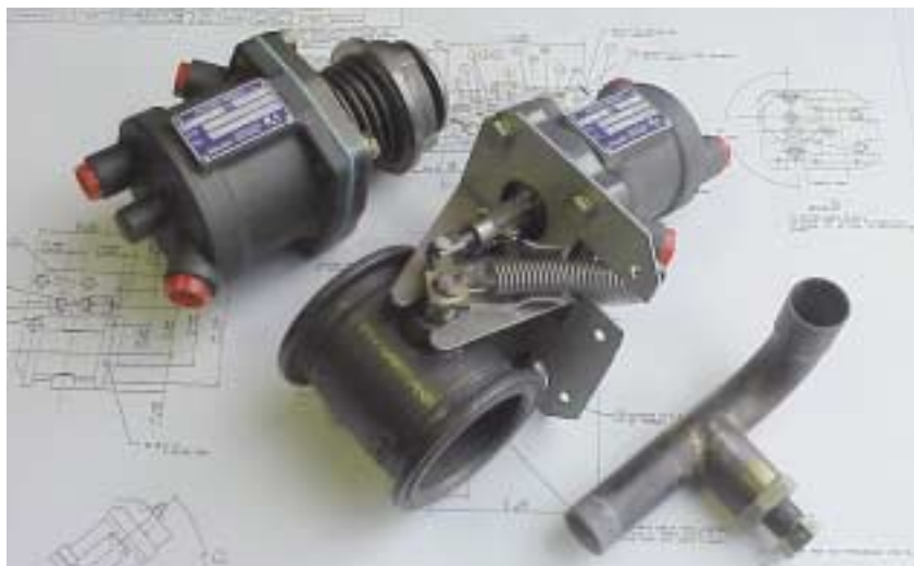
Exhaust bypass valves: butterfly, poppet and fixed. Note that Continental's "fixed" wastegate system relies on an adjustment screw in the turbine bypass pipe (right). Ground adjustments are made by loosening the lock nut and turning the screw into or out of the wastegate bypass pipe.
