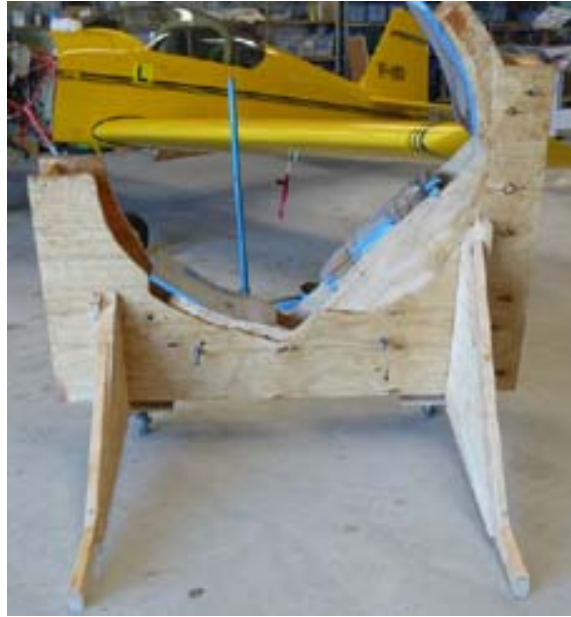
Front of fuselage stand, level and rear side rotated
