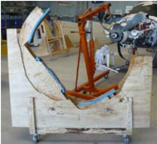
Fuselage stand front rotated and with rear side with rotator cradle removed
