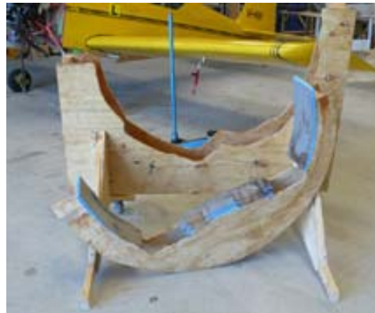
Fuselage stand front rotated and with rear side with rotator cradle removed
