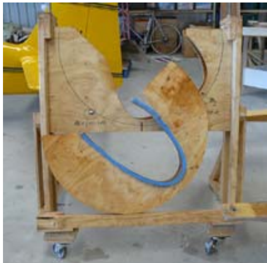
Back side of rear fuselage stand rotated, and rotator cradle removed
