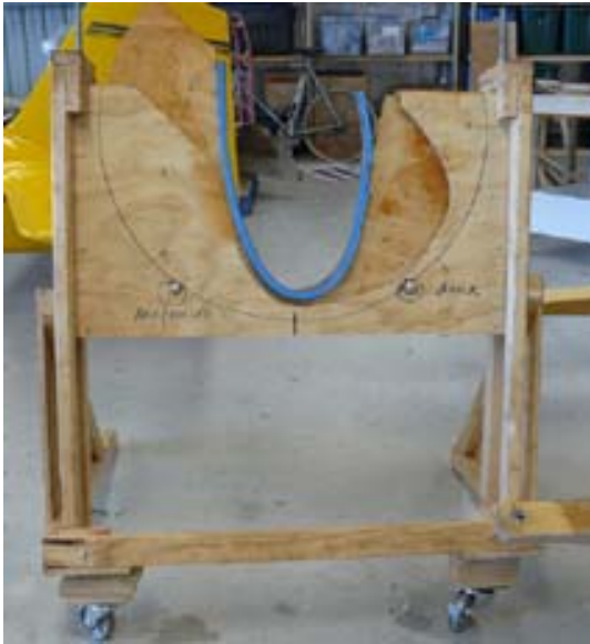
Fuselage tail stand with vertical adjustment, vertical and rotated positions
