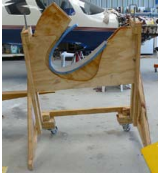
Fuselage tail stand with vertical adjustment, vertical and rotated positions
