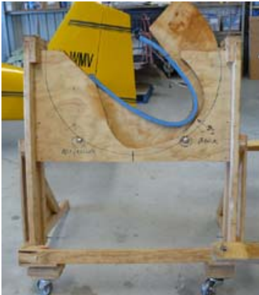
Back side of rear fuselage stand rotated, and rotator cradle removed
