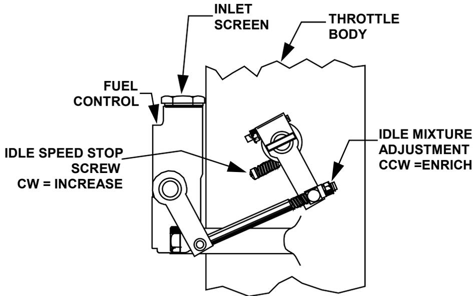
**FIGURE 9 - THROTTLE & CONTROL ASSEMBLY
