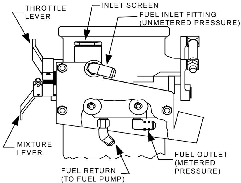
**FIGURE 7 - THROTTLE & CONTROL ASSEMBLY - FRONT VIEW (EXCEPT GTSIO-520-D,F,H,K,L,M,N)**
