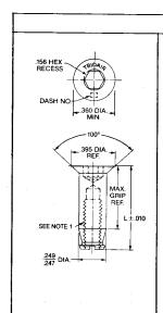
100° C'Sink **Hex Recess** Material Part No. Material: 300 Series CRFS CA1820-( ) Finish: Passivated per QQ-P-35 Material: 300 Series CRFS CA1820-( ۱B Finish: Black Oxide per MIL-C-13924 Material: 300 Series CRES Finish: Cadmium Plated per QQ-P-416. CA1820-( )C Type II, Class 2 Material: Allov Steel Heat Treat: Per MIL-H-6875 Finish: Cadmium Plated per QQ-P-416, Type II, Class 2 Material: A-286 CRES Heat Treat: Per MIL-H-6875 CA18187T-( Finish: Passivated per QQ-P-35
